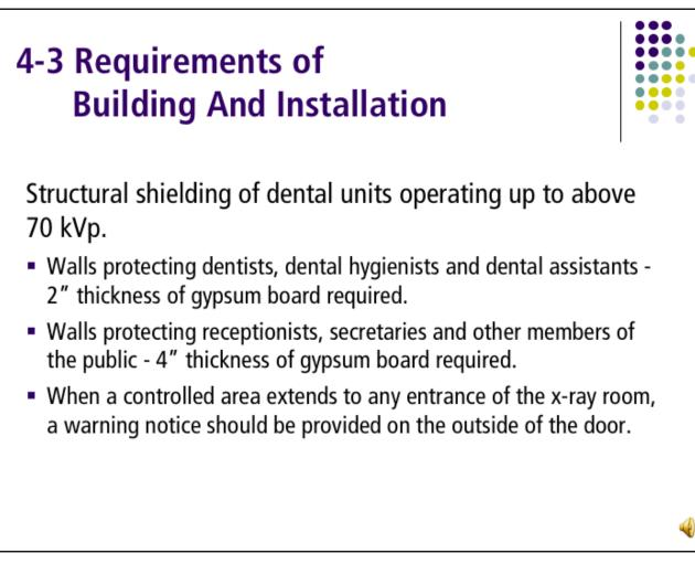
Examples of Building and Installation Requirements: Structural shielding of dental units operating up to above 70 kVp.
