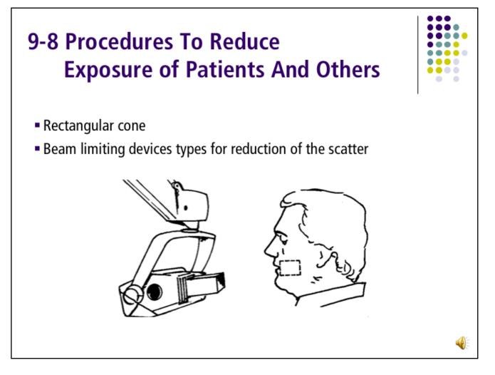
It is recommended that rectangular collimation be provided on new equipment and be retro-fitted to existing equipment at the earliest opportunity. Rectangular collimators should be designed so that the beam size at the end of the collimator does not exceed 40 by 50 mm.
