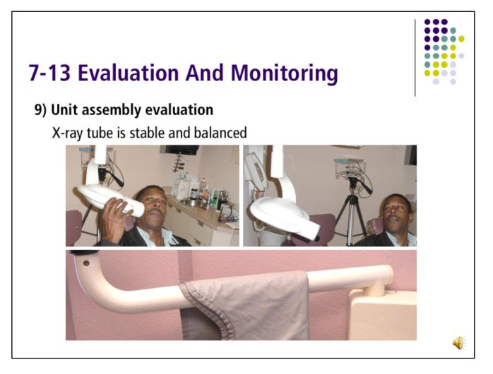
**Unit Assembly:** Both mechanical and electrical stabilities must be within the manufacturer's specification. The X-Ray tube housing must maintain its required position or movement without excessive drift or vibration. Otherwise service is recommended.
