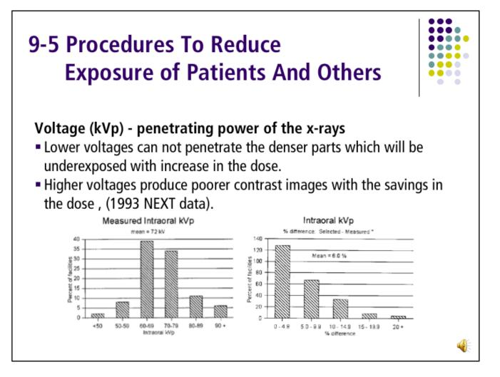
Dental radiography must not be carried out at X-ray tube voltages below 50 kilovolts (peak) and should not be carried out at X-ray tube voltages below 60 kilovolts (peak).
