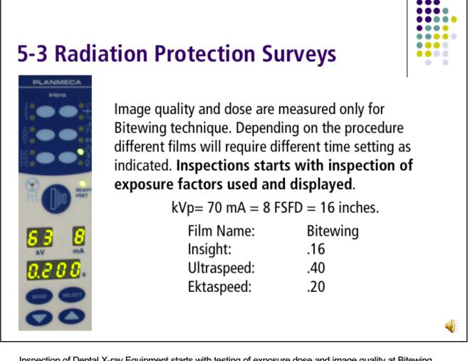
Inspection of Dental X-ray Equipment starts with testing of exposure dose and image quality at Bitewing exposure technique. Equipment is than tested for linearity performance at all combinations of exposure factors used. Image quality and dose are measured only for Bitewing technique. Depending on the procedure different films will require different time setting as indicated in the table.
