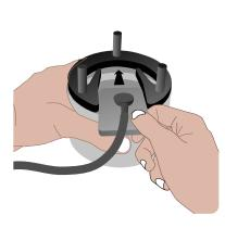
Slide the sensor in the black sensor holder with the cable connector on top as shown in the drawing on the left.
