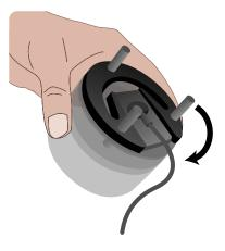
Flip phantom with sensor detector installed over and place on a flat, stable, horizontal surface.
