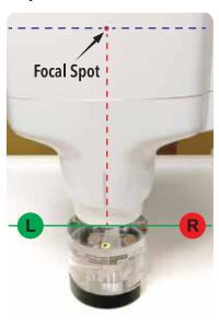
Please check you dental x-ray unit and determine where there is a "dot" of your system indicating the anode location. This should be aligned with the "F" label on the phantom.
