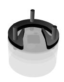
Place the phantom on a stable horizontal surface with the black sensor holder on the top side.
