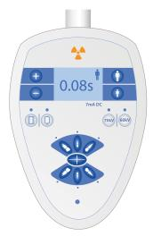
Select the setting for bitewing exposure (for the example provided a 0.08s is selected). Create a patient file for Quality Assurance before you press exposure. Store your phantom images in this file for reference and comparison over time.
